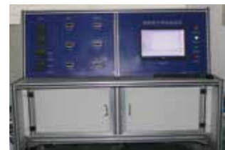
碳刷试验控制柜 Carbon Brush Testing Control Cabinet
