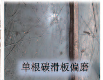
single carbon contacts Partial wear
